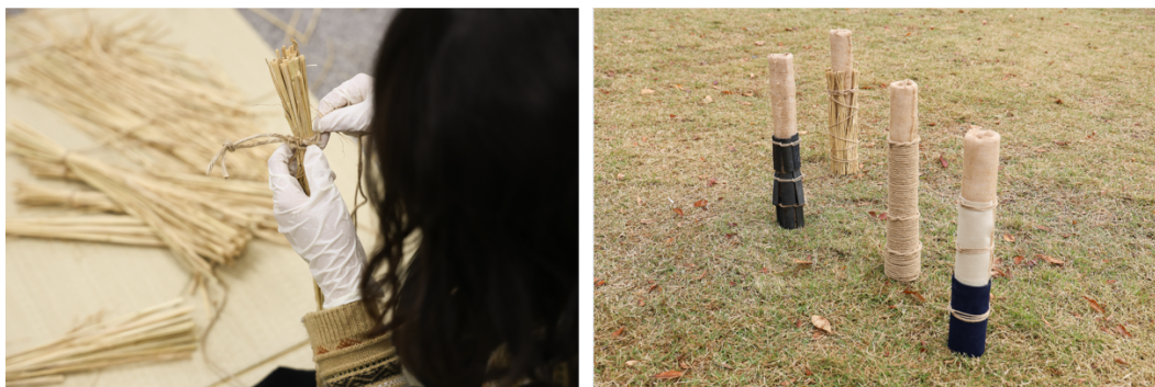
Figure 6. Fabrication Process and Finished Product of the Third Prototype. Materials used included Carbon Sheet, Straw, Hemp Rope, and Felt.
